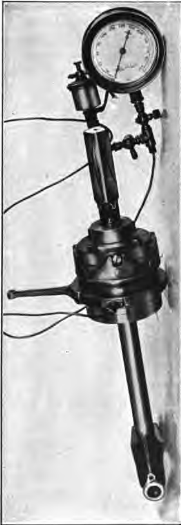
Fig. 94.—Transmission Dynamometer in Automobile Propeller Shaft, 30 H. P. at 500 R. P. M., Weight 25 lb.
